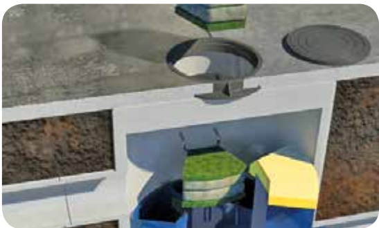
Fig.4b Media bags are replaced manually with no heavy lifting equipment required.
